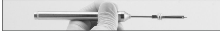
2. Now the screwdriver with claw is ready to use. To secure a screw, push the claw ② in the direction of the screwdriver blade over the screw until it snaps into groove 2 (④, closed position). For Disassembly push and remove the claw ② into the direction of the screwdriver blade.
